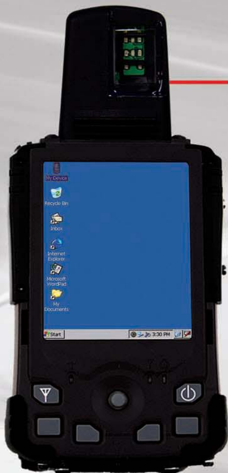
500 dpi Optical Scanner Detail
